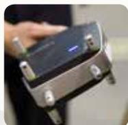
**T-Scan CS.** Hand- held 3D digitizing system with laser/optical technology. The revolutionary and modular all-in-one concept, includes perfectly matched components (tracking camera, hand-held scanner and touchprobe), thereby
